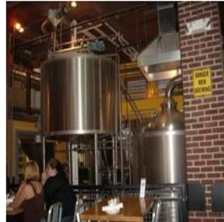
In the kettle, the wort is boiled for an hour and 15 minutes and varying amounts of hops are added to give bitterness, flavor, and aroma characteristics. After the boiling process, the wort needs to be prepared for fermentation, so a counter-flow heat exchanger (using glycol and city water) is used to cool it down to 65°F. Oxygen is also infused into the wort at this point to help with yeast respiration.
